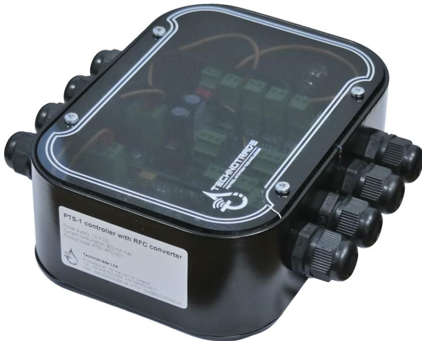
Variant of RFC interface converter supply installed in a mounting box together with PTS-1 controller in a plastic box with cables inputs and power switching button (RFC-PTS-z)
