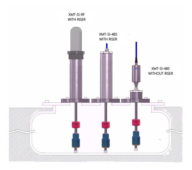
Please follow the above procedures if probes are wired. The only difference is that the length of the riser must cover the total length of the probe, and a cap with a cable gland must be screwed to allow the exit of the connection cable.
