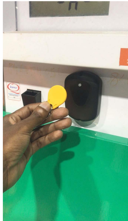
Example of reader installation on fuel dispensers
