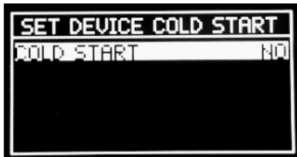
Cold start can be also done using buttons S1 and S2 on the board. For cold start hold both S1 and S2 buttons during the power on of the U2L converter for at least 5 seconds.
