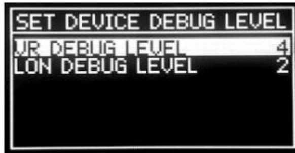
Adjust device debug levels. These parameters are used only for service purposes during logging and do not affect the normal communication of U2L with the other devices. Below the parameters included in the menu:
