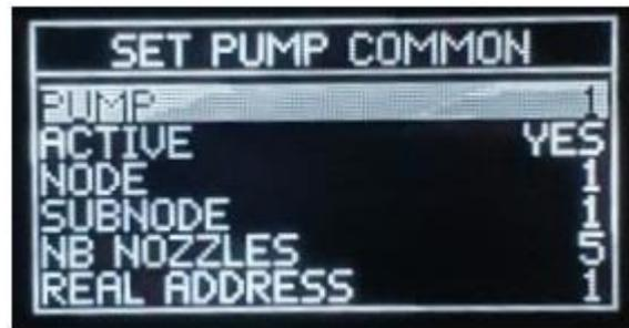
This sub-menu arranges the relation between the fuelling dispensers (pumps) on the field, their filling positions (FPs) and the addresses assigned to them.
