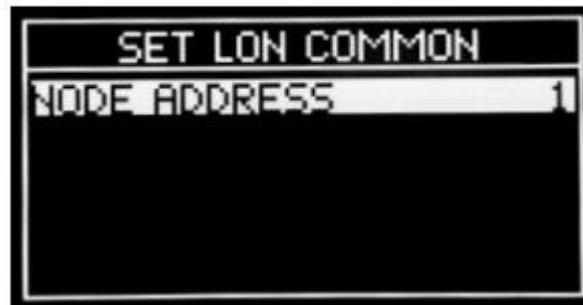
Set the LON-network node address. It is important to make sure that the device is set with a unique address in the connected LON-network. From pumps prospective the U2L-bridge appears as POS-system and its node-address.
