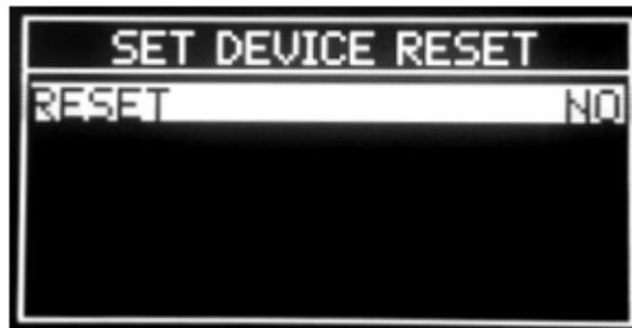
Device reset. For activating the reset press OK and then by UP/Down keys select 'YES' and then push OK button. The reset is executed when quitting this menu.
