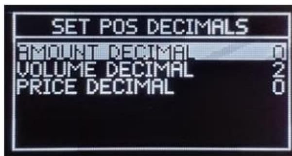
The below menu specified the decimal position of the following parameters:
