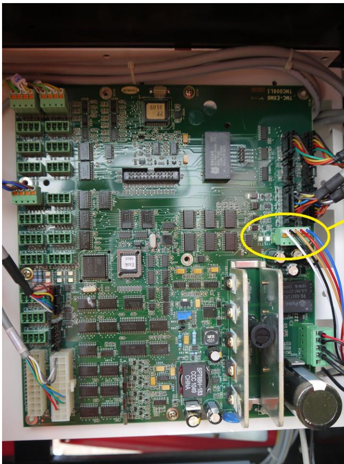
Tokheim dispenser calculator with interface board
