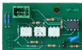
Nuovo Pignone interface boards for RS-485 interface for monoproduct and multiproducts dispensers
