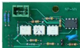
Nuovo Pignone interface boards for RS-485 interface for monoproduct and multiproduct dispensers
