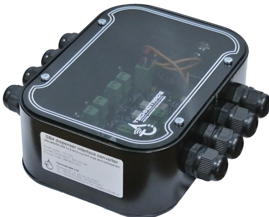
Variant of GB-4 interface converter supply installed in a plastic box with cables inputs and power switching button (GB4-BOX-z)
