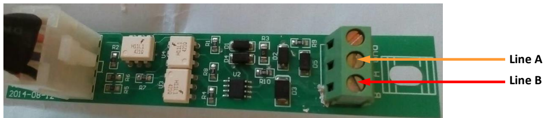
Datian Machines dispenser interface board
