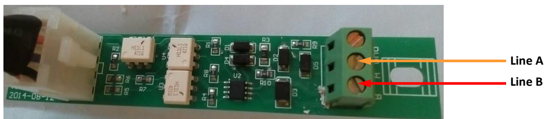
Datian Machines dispenser interface board
