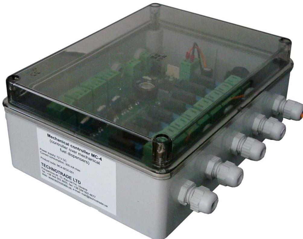
Variant of MC-4 controller supply installed in a plastic box with cables inputs and power switching button (*MC4-BOX-z*)
